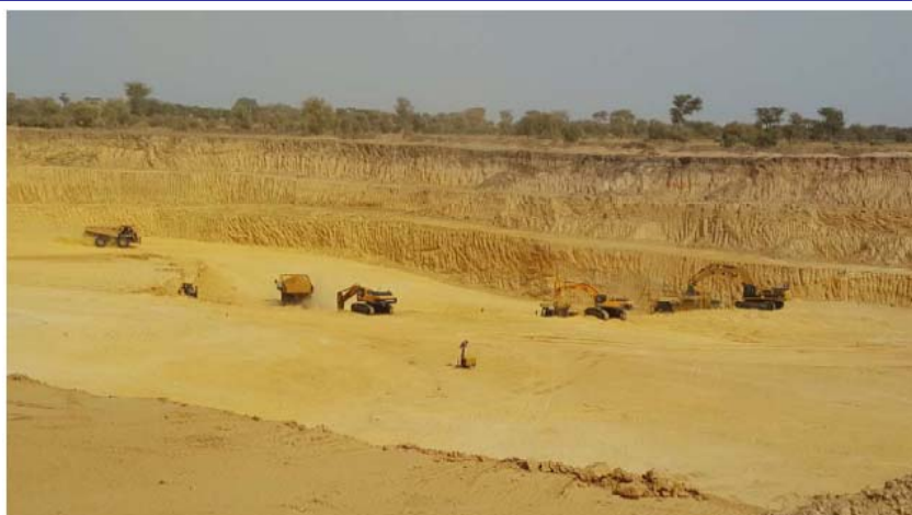
Figure 1 : Over-burden removal progressed
