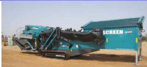
Figure 4b : Wet plant screen feeding unit
